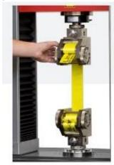
Note 5: The use of clamps for testing reinforced tapes is discouraged because the strength of reinforced tapes requires excessive clamping pressure which can cause crushing of the reinforcing filaments. When this occurs, the tape usually breaks at the jaw edge which can result in lower breaking values. Hence the use of cylinders described in 5.1.3 is recommended for reinforced tapes.
